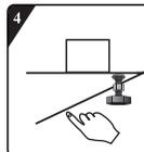
Press the double sided tape on four sides manually to secure the noise-reduction palte to the machine body firmly.
