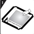
Before installing the noise-reduction bottom plate, align and paste the acoustic absorption wool with and along the right-angle impression on bottom plate (this procedure is unnecessary for some of the models without acoustic absorption wool).
