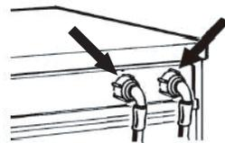
10 Screw by hand the inlet hose onto the tap, tightening the nut.
