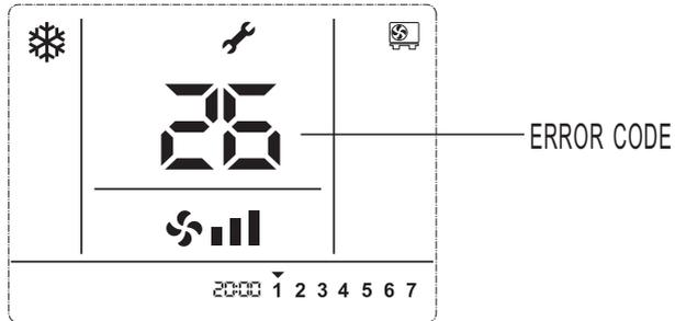
When the airconditioner is malfunction,
