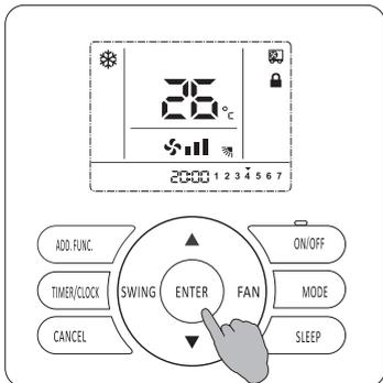
After wire remote controller setting is finished, you can set button locked function to avoid children or other people's wrong operation. All operations are invalid after button locked function has been set.
