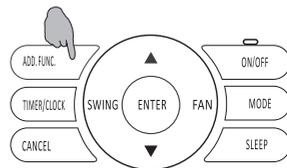
After manually set the electric heater on, the indicator will lights on, and will light on/off according to the actual state after 5 minutes (electric heater may not start as the internal control condition is not satisfied).
