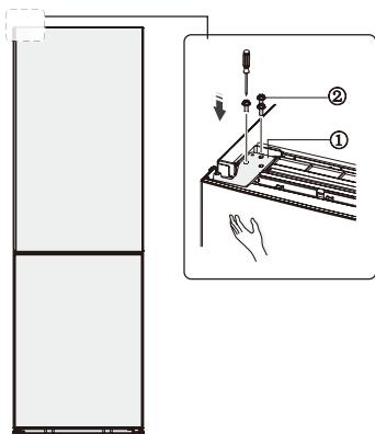
16. Reverse part① by 180°and install it onto the right corner of upper door, then mount part②. (both of which are taken down in step 2)
