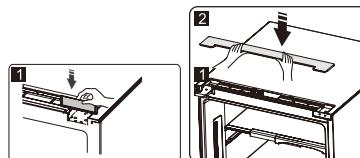
15. Install part the upper hinge cover(which is in the plastic bag).
