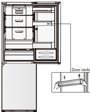
2. Open part ① on top of the refrigerator body from right side and then take down part ③ and part ④ on the upper door in the same way. Take down part ② and put it back to the plastic bag.
