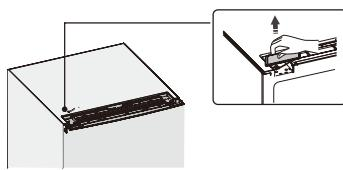
4. Remove the screws ① , and remove part②.
