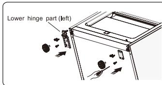
12. Move the lower door and adjust its position to align lower hole site and upper hinge axis. Turn the middle hinge by 180, change the washer on the axis to the upper side, adjust the middle hinge to the appropriate position and then install it.
