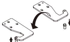
14. Move the upper door to appropriate position, adjust part① and upper door, then fix part① by screws②. (Please hold upper door by hand when installing)
