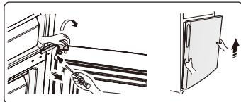
7. Place the lower door on a smooth surface with its panel upwards. Loose screws③ , detach part② and part① . Turn part①by 180°and then install ①and part②to corresponding position on left side together with screws③.
