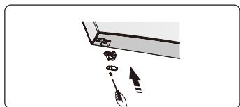
8. Change screw hole covers on middle cover plate from left to right (as shown in figure below).
