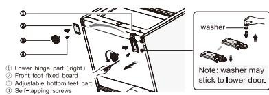
10. Screw out lower hinge, change it to the near hole site, and then screw up and mount washer.
