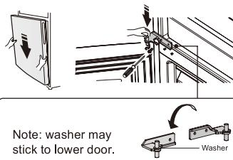
13. Screw out The upper hinge axis, turn the upper hinge over and fix axis on it. Then place it at side for use.
