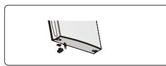
6. Loose screws used to fix the middle hinge and remove middle hinge. Then remove the lower door.
